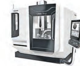
DMG MORI CMX 70U 5 Axis VMC 800 X 560 350 kg loading capacity 5 pieces
