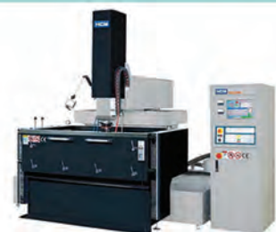
HCM HC1060 +300 HIGH 5 Axis EDM 1250 x 750 4.5 tons loading capacity
