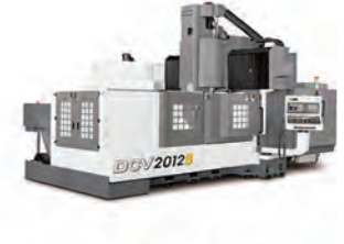
YCM DCV 2012B 3Axis VMC 2000x1100 5 tons loading capacity 2 pieces
