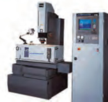
JOEMARS P50 4 Axis EDM 600 X 300 500 kg loading capacity
