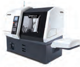
DMG SPRINT 32/8 8 Axis Horizontal Production Turning
